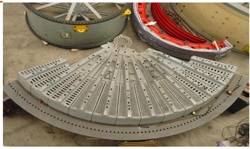
Trial Installment of mill liner
