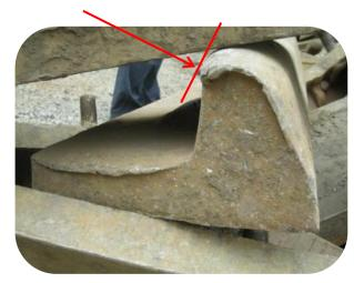
Poor Design :Liner Yield Deformation by Direct Smash of Balls Due
