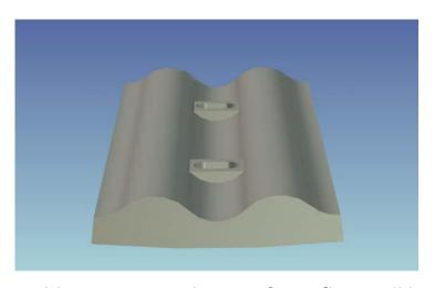
Double wave crest design of overflow mill liner
